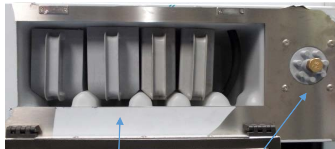
Detergent compartments and connection to dosing pumps
